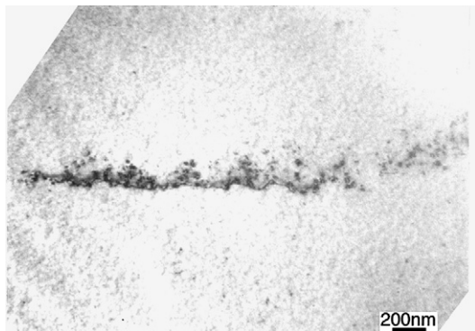
Fig. 5. Decoration of edge dislocation by interstitial type dislocation loops in Fe irradiated at 473 K to 0.061 dpa.
